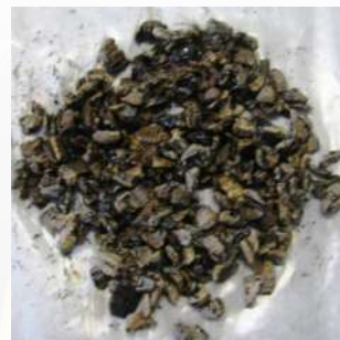
Aggregates: Bitumen without Antistripping agent, after Boiling Test.
