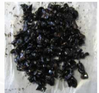
Aggregates: Bitumen with Antistripping agent, after Boiling Test.
